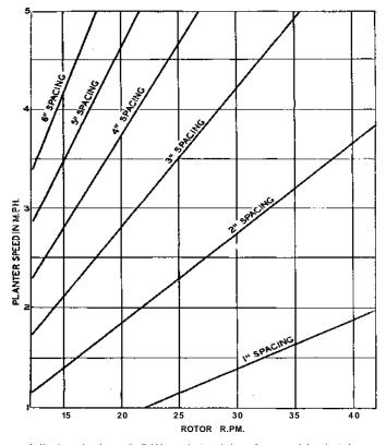
Indications size that each Cobbley unit (consisting of rotor and housing) has an optimum rotor rp.m. at which optimum speed it dispenses approximately 100 seeds per 100 cells and causes the least damage to the seed. When this optimum rotor r.p.m. has been determined for an individual Cobbley unit and the desired seed spacing is known, the correct planter speed in in.p.h. for the optimum rotor speed can be determined from the chart shown hero.
