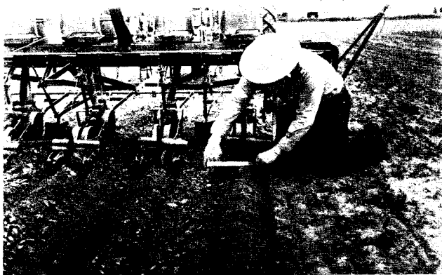
Figure 4.—A pair of small disks, weighted to improve penetration, was used at the rear of each furrow opener for the covered-row planting.
