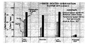
Curve No. II.—Shown here is the reduced efficiency of the combination through increased ground speed. It will be noted that the curves level out at about 62 percent which shows that the beater becomes ineffective at that point and the remaining beets topped are those topped by the knife unit.
