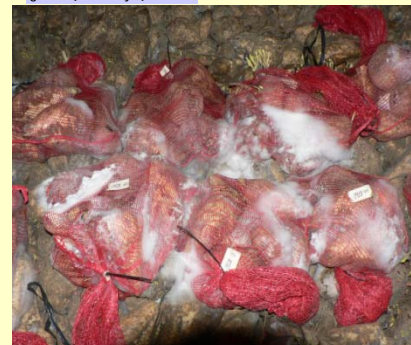
ON pile samples with fungal growth (basidiomycete)
