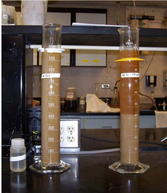
Figure 2. First Carbonation Juice Without and with starch addition after 1 minute of settling.
