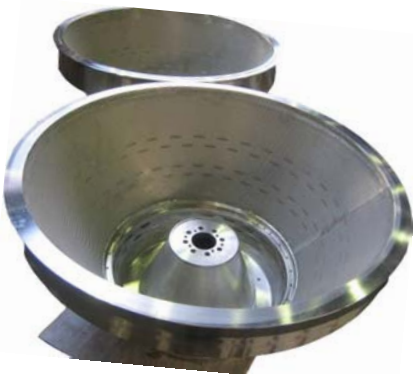
Fig. 1: Newly designed two-stage basket
