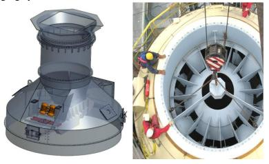
Mechanical design and operation capabilities of hydraulic driven discharge equipment with its volumetric material movement. Review of the advantages in production and process in shaft kilns. Successfully implemented at Michigan Sugar - Bay City in 2016.
