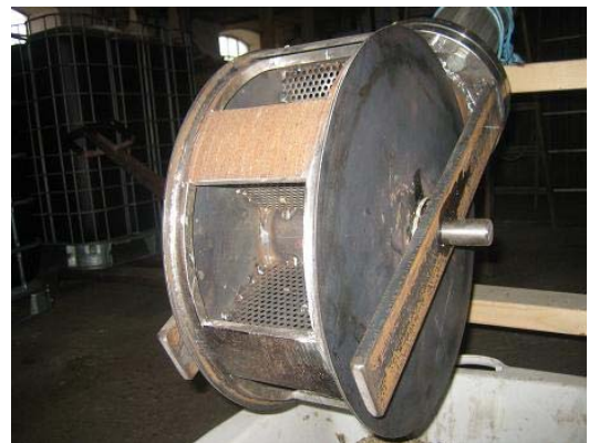
Fig. 10, valve for discharging pulp. Chambers are made of perforated plates.
