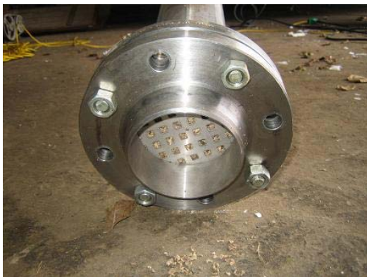
Fig. 9, perforated plate is holding back the pulp.
