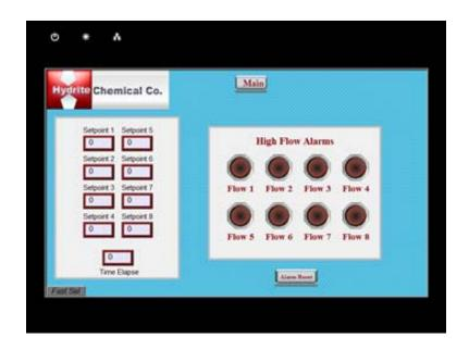
Set points can be configured with time limits to notify the plant that the flows have been set to high for too long and that their attention is needed. These alarms can be sent via text messaging or emails
