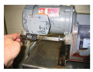
(Use Digital Calipers to Set Pump Rates)
