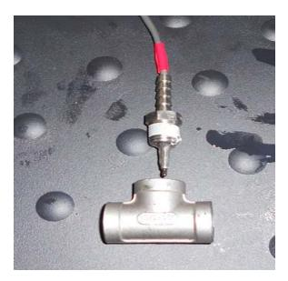
The flow sensors are manufactured in a 2 piece stainless steel configuration. The solid state sensor is mounted in epoxy in a stainless steel threaded bushing. The sensor is threaded into the stainless steel tee. This makes for easy installation and replacement.
