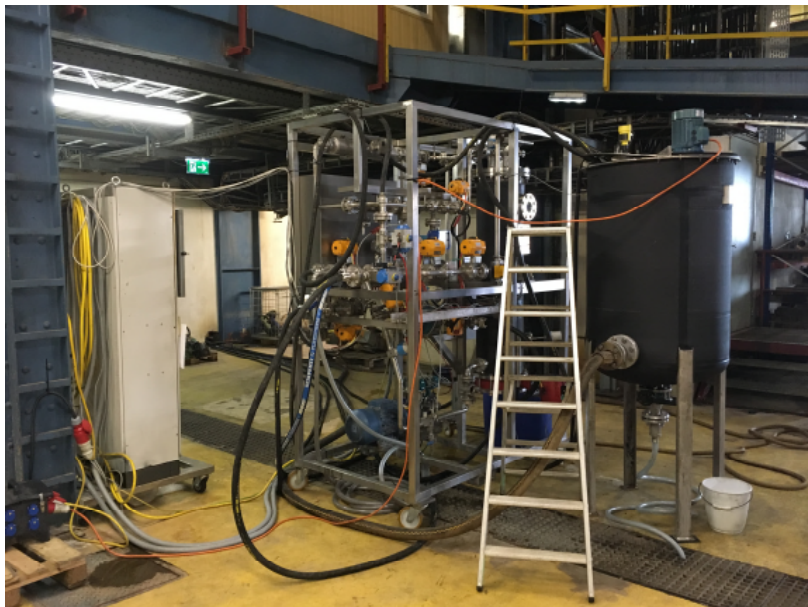
Figure 17: Pilot unit Lenzing CakeFil in operation
