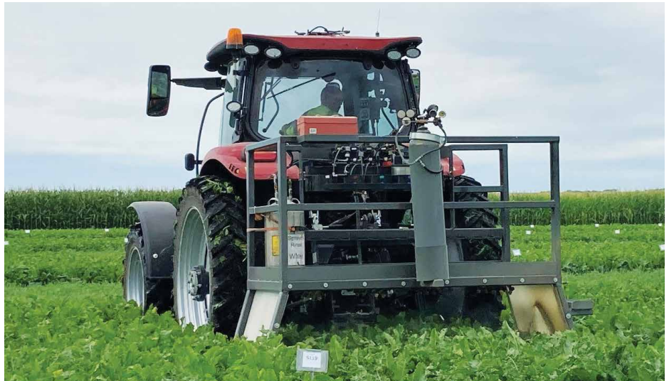
Photo 1. Tractor mounted hooded sprayer used to apply fungicide treatments.
