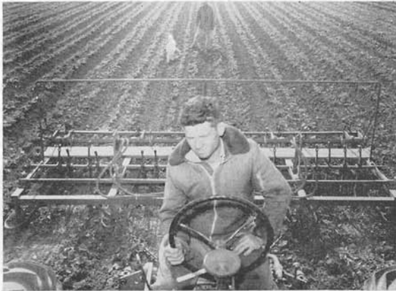
Figure 8.—1957—The second and subsequent cultivations by the Collier sled required no accurate tractor steering; the sled runners followed the original furrows and gave accurate lateral positioning of cultivator tools.
