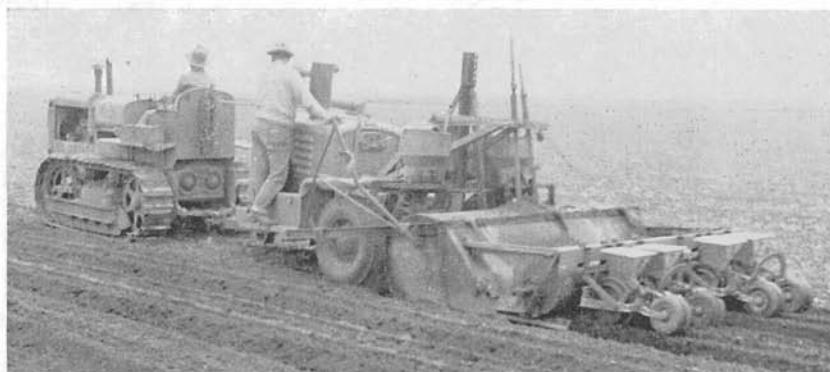
Figure 2.—1948—K. B. Fiske of Woodland, California, combined a Sea-man Tiller, John Deere fertilizer applicator, listing shovels, bed roller, and Milton panter.
