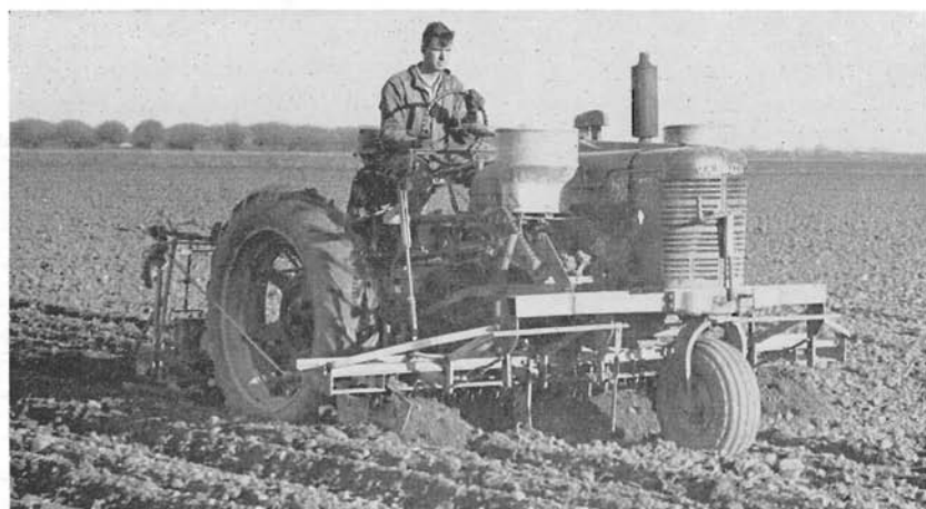
Figure 1.—1947—Jaeger & Stevens of Madison, California, equipped a tractor for listing, bed shaping, and planting in one operation.
