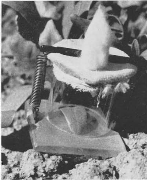
Figure 1.—Clip cage used to confine beet leafhoppers on test plants. (Actual size \frac{3}{4} inch diameter.)
