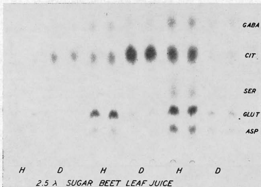
Figure 1.—Papergram, developed in water-saturated phenol, of juice expressed from mature leaves of 3 healthy plants and juice from leaves of comparable age from 3 plants having yellows showing. Aspartic acid (asp.), glutamic acid (glut), serine (ser), citrulline (cit), and -aminobutyric acid (gaba). Other amino acids are present with r-aminobutyric acid. H-Healthy leaf, D-Diseased leaf.
