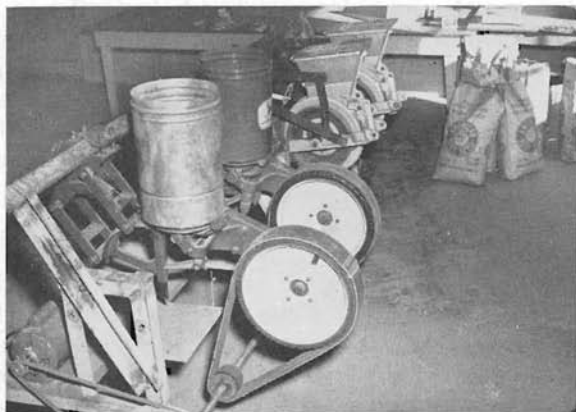
Figure 1.—Picture of drill test rack mounted with units of three makes of drills used in experiments at Rocky Ford, Colorado.
