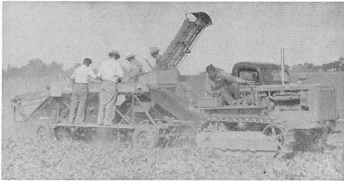
Figure 12.—In 1941 Austin Armer, University of California, developed this two row beet harvester, using the hand-sorting principle suggested by Prof. Roy Bainer.
