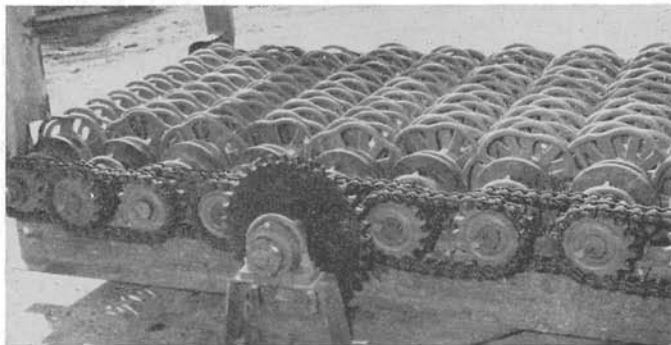
Figure 11.—The now famous Rienks Screen was developed by Mr. George Rienks, Sr., based on the star wheel principle.
