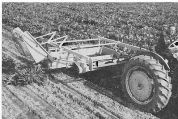
Figure 6.—The Wescon topper, like the Lockwood and Speedy, delivers multiple windrows of beet tops (1964).
