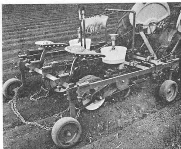
Figure 3.—Fully assembled seeder showing attendant seating, seed envelopes arranged on wire rods, and sprocket arrangement for sowing a 53-foot plot.
