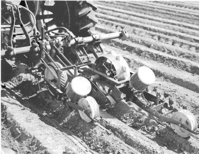
Figure 10.—Field unit used in 1971 emergence and planting date comparisons. The left planter is a John Deere No. 33 vegetable planter, and the right planter is the Wyoming (or Jafari) space planter.
