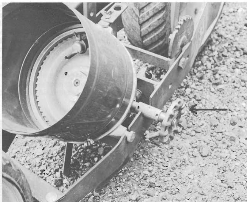
Figure 2. —Steam valve handle installed on right end of seed hopper shaft for manually turning seed plate.
