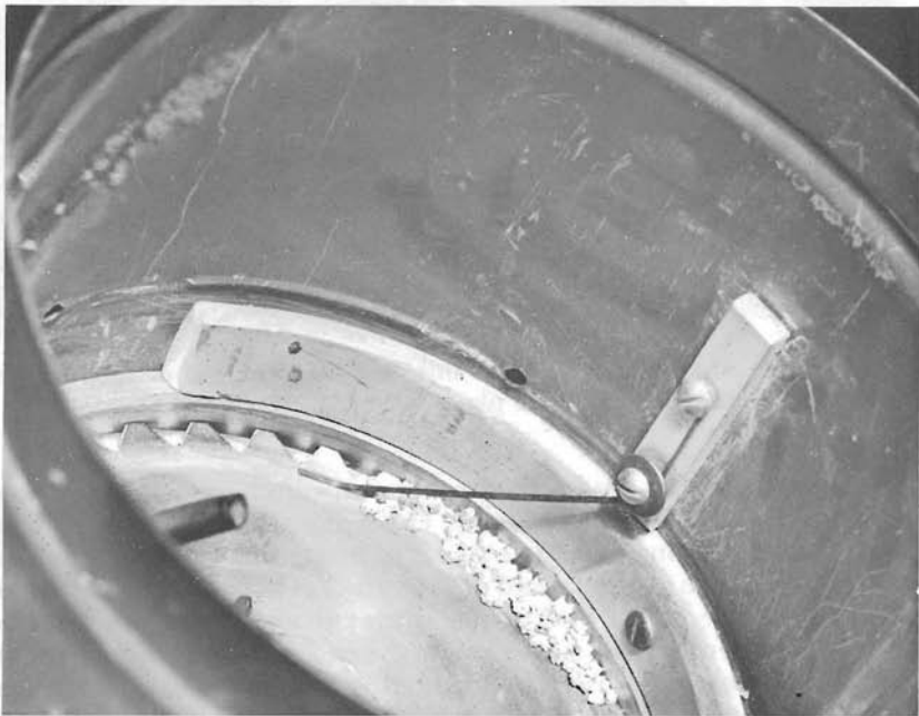
Figure 1. —Metal tine installed in seed hopper to deflect excess seeds to bottom of hopper.
