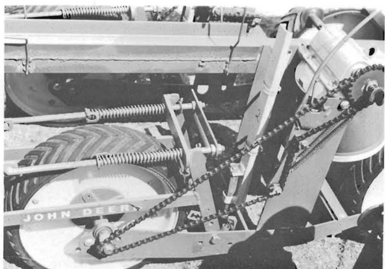
Figure 1.—(Top). Modified planter assembly in operating position; A: steel disc welded to hopper shaft to serve as a handle to turn the planter plate when the driven sprocket is disengaged; B: lever used to disengage driven sprocket; C: steel plate used to support the hopper about 14 inches above the original site.
