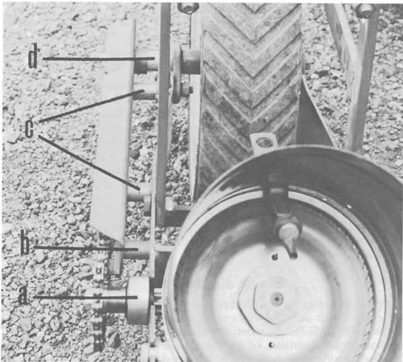
Figure 3.—One-way overriding clutch installed on John Deere Model 33 vegetable planter unit. a - Bendix starter drive; b - spacer for chain tightener; c - spacers for chain guard; d - machined spacer for drive wheel sprocket.
