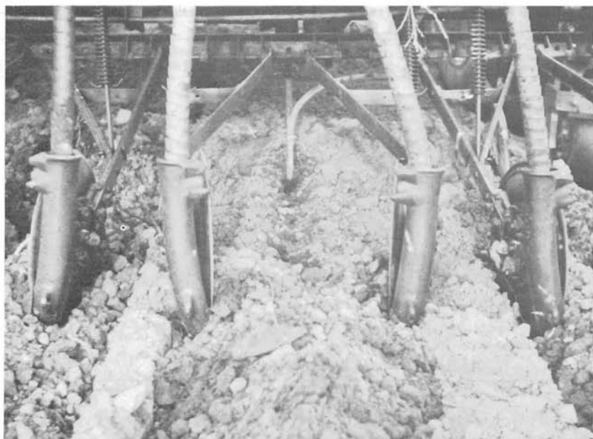
Figure 1. — Close-up converted grain drill used to apply starter fertilizer, form a small bed and sow barley adjacent to the future sugarbeet row.
