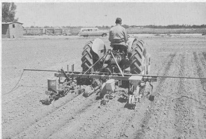
Figure 7.—General view of some of the beet planters used in the 1955 field test. Left to right the planters are Ventura, Stanhay, Semora and Milton.
