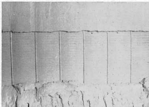
Figure 6.—4-inch spaced wrap on rubber grid equipped filter.
