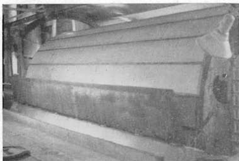
Figure 1.—General view of Plaste coated vacuum filter (perforated screen grids).
