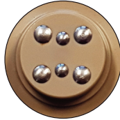
Figure 8. Conductivity Electrode Designs. A four pole with 6 electrodes shown below.
